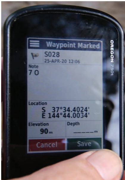
Figure 3: Collecting GPS data GPS recording unique warren ID S028, number of burrows (7) and activity (O=open)
